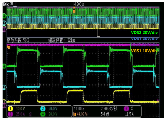
Figure 14. Operation in 2kW LLC Converter
